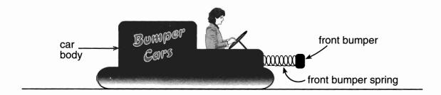
On one occasion Petra's car hits a rigid wall and the bumper becomes stuck fast to the wall. This leaves the car oscillating horizontally with simple harmonic motion (SHM) for several periods. Under these conditions the car can be modelled as a single point mass, at the centre of mass of the car, performing SHM on the end of a horizontal spring as shown below.
