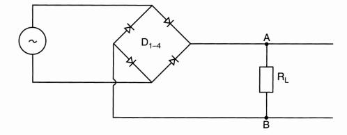
(g) At certain speeds of the car, the frequency of the AC electricity produced is 75 Hz. On the axes provided in your Answer Booklet, sketch a graph of the voltage across AB against time for two full cycles of the generator. Include numerical values for both voltage and time, but ignore any voltage drop across the diodes.
