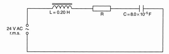
The frequency of the source is adjusted to the resonant frequency of the circuit.
